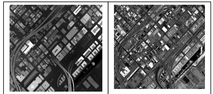
Figure 2: Lidar Data ( Left Image Shows Lidar Height Data and Right Image Shows Lidar Intensity Data)
